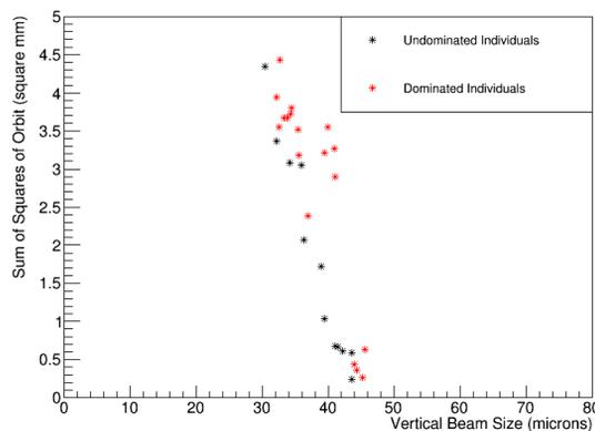
Figure 3: Population in data after 10 generations when using the first 8 eigenparameters as our genes.
