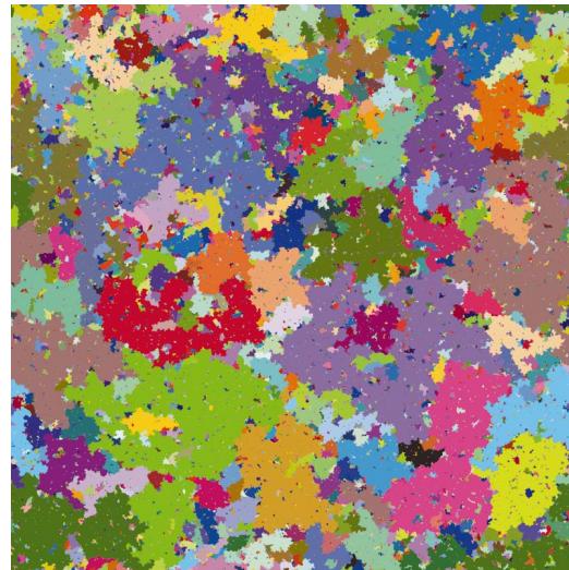
Figure 4. A 30,000 \times 30,000 simulation with disorder R = 0.65 , where each pixel represents a 30 \times 30 square, and each avalanche is a different color. There are avalanches of all sizes, with many smaller avalanches and fewer large ones.
