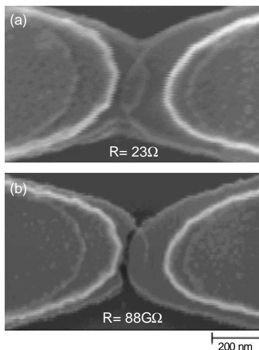
Fig. 1. Field emission scanning electron micrographs of a representative gold nanowire (a) before and (b) after the breaking procedure described in the text. The nanowire consists of thin ( $\sim 10$  nm) and thick ( $\sim 90$  nm) gold regions. In the images, diffuse white lines separate these two regions.
