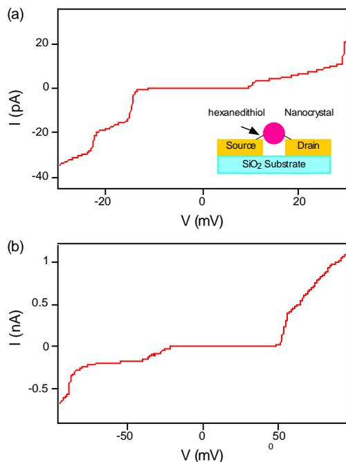
Fig. 3. Current vs. voltage curves at  $T = 1.5$  K obtained from single electron transistors based on (a) 5 nm CdSe nanocrystals and (b) 7 nm CdSe nanocrystals. The inset in Fig. 3(a) shows the schematic diagram of an idealized device.
